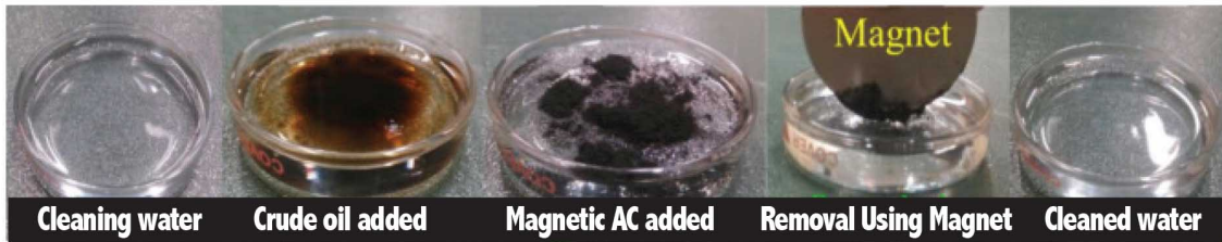
Demonstration of crude oil removal in water using the developed magnetic carbon product.
